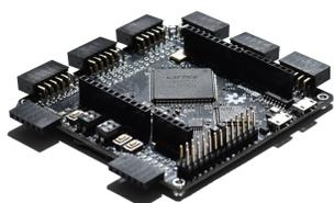
Figure 2.1: The BlackIce II board and Lattice iCE FPGA.
